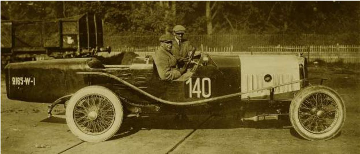
*Designed by the boss himself and build in a few days to be entry in hill-climb competitions, the car has a standard 4 litre sleeve valve engine modified with lightweight aluminium pistons and tubular connecting rods, delivering nearly 100 bhp at 2,950rpm.*
